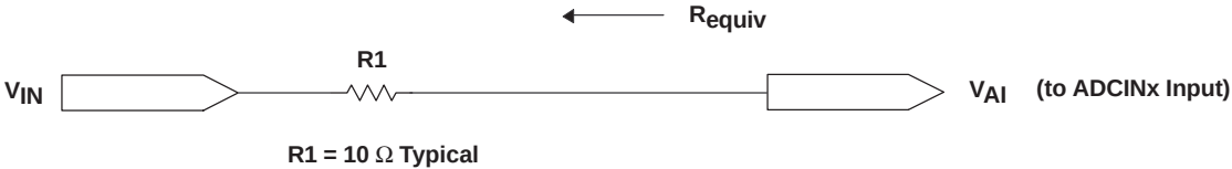
Figure 41. Typical ADC Input Pin Circuit
