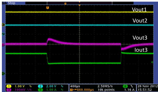
Figure 24. Transient Response Buck3@3.3V, 1-2A Step, C_o = 22\ \mu\text{F}
