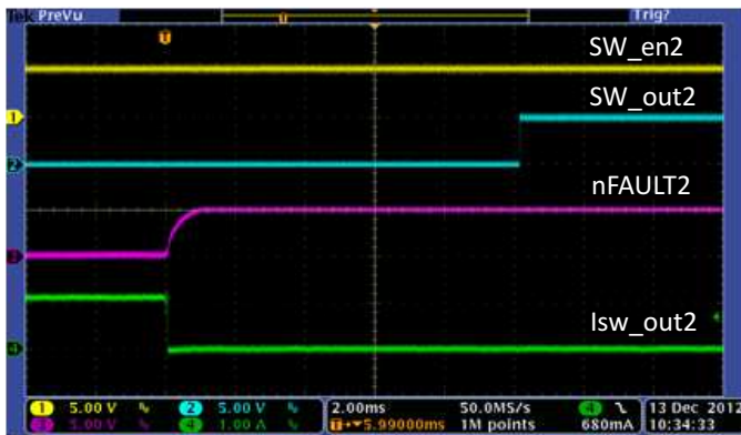
Figure 44. USB Switch2 Current Limit Recovery
