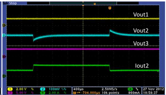
Figure 23. Transient Response Buck2@1.8V, 1-2A Step, C_o = 47\ \mu\text{F}
