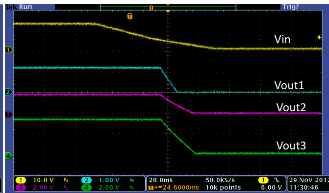
Figure 17. Power-Down All Converters, No Load
