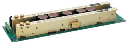
Fig. 58 Backplane for system integration
