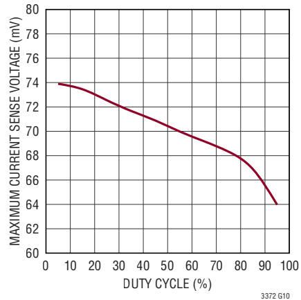
Maximum Current Sense Threshold vs Duty Cycle
