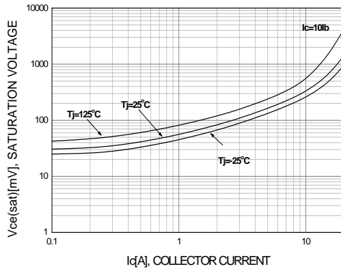
Figure 4. Collector-Emitter Saturation Voltage
