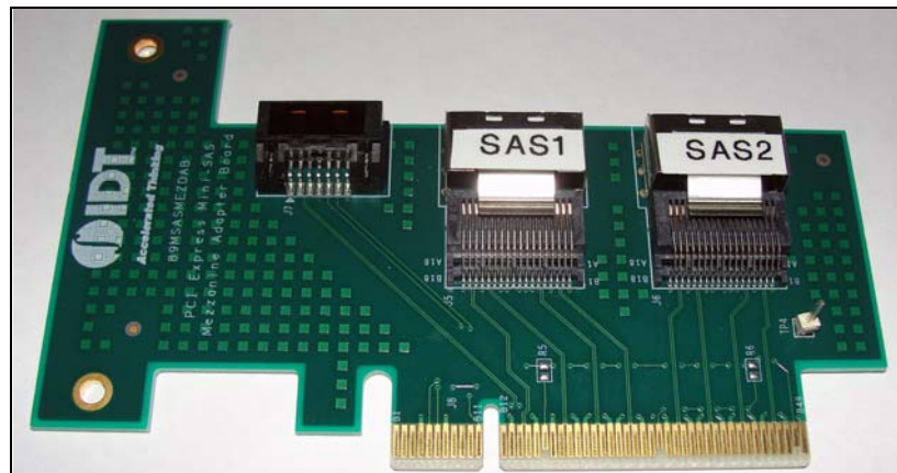
Figure 2.6 PCIe x8 Edge-to-SAS Adapter
