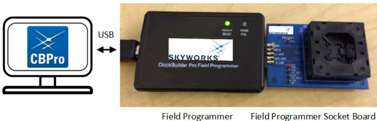
Figure 14. Connections from PC to the Target Device
