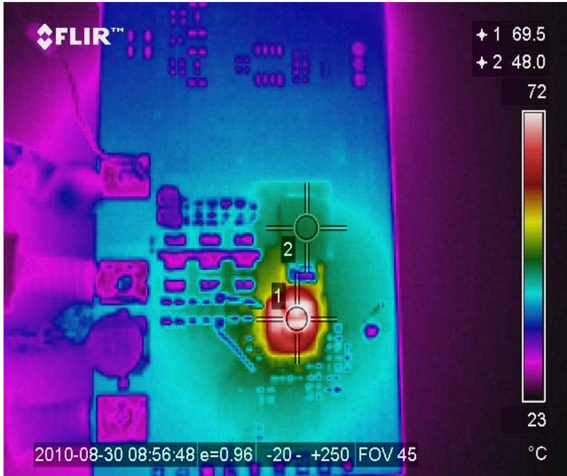
Figure 31: Thermal Image of the board at 35A load Test point 1 is iP1837 Test point 2 is inductor
