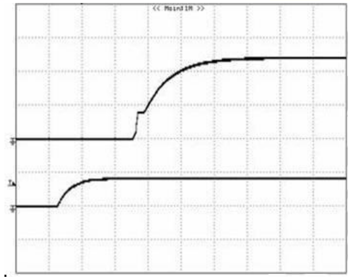
Figure 6: (For positive remote on/off logic) Turn-on transient at full rated load current (5 ms/div). V_{in}=48V . Top Trace: V_{out} , 5V/div; Bottom Trace: ON/OFF input, 5V/div.
