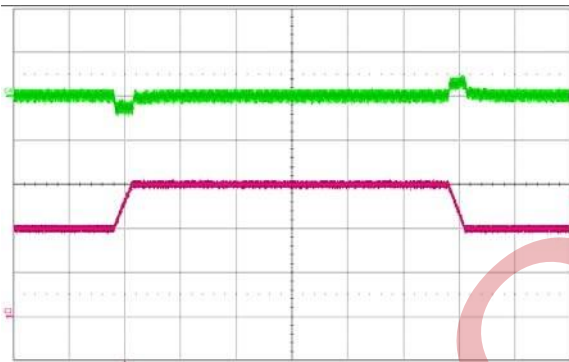
Figure 11. Output voltage response to load current step change (10A – 15A – 10A) at Vin = 48 V. Top trace: output voltage (50mV/div.) Bottom: load current (5 A/div.). Current slew rate: 0.1 A/us. Time scale: 200 us /div. Co = 10uF tantalum + 1uF ceramic
