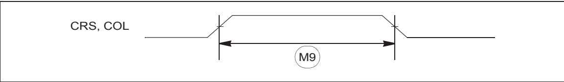
Figure 41. MII async inputs timing diagram
