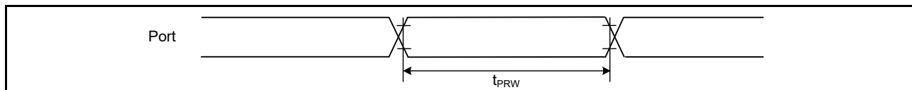
Figure 2.28 I/O ports input timing
