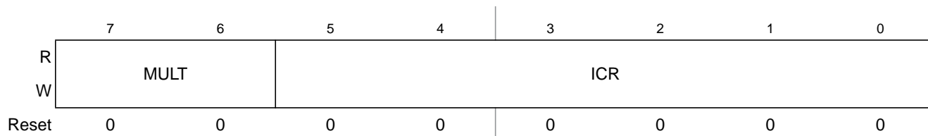
Figure 11-4. IIC Frequency Divider Register (IICF)
