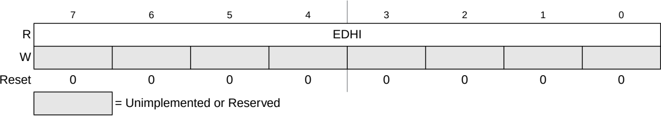
Figure 25-15. EEPROM Data High Register (EDATAHI)
