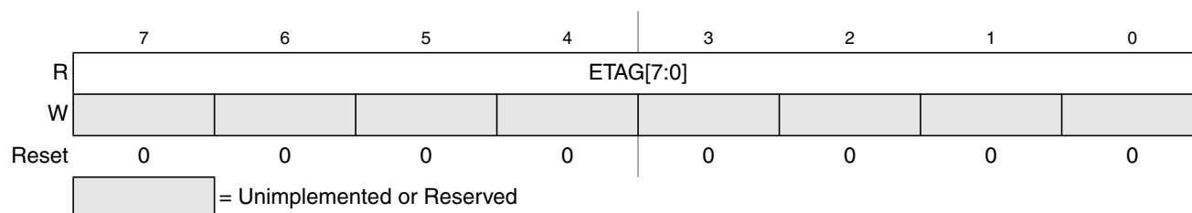
Figure 24-19. EEE Tag Counter Low Register (ETAGLO)
