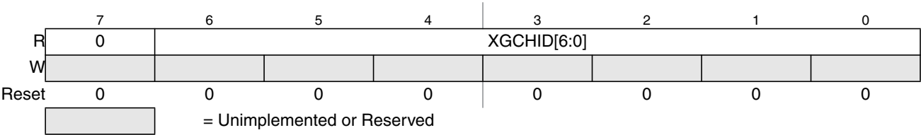
Figure 10-4. XGATE Channel ID Register (XGCHID)
