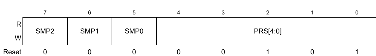
Figure 12-7. ATD Control Register 4 (ATDCTL4)
