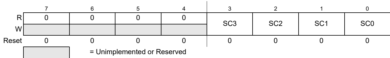
Figure 8-9. Debug State Control Register 1 (DBGSCR1)
