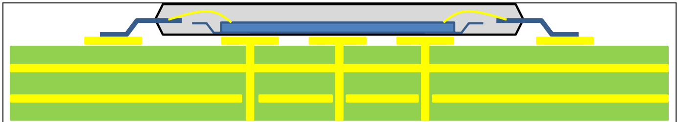
Figure 8-1: Example Thermal Via Holes on PCB
