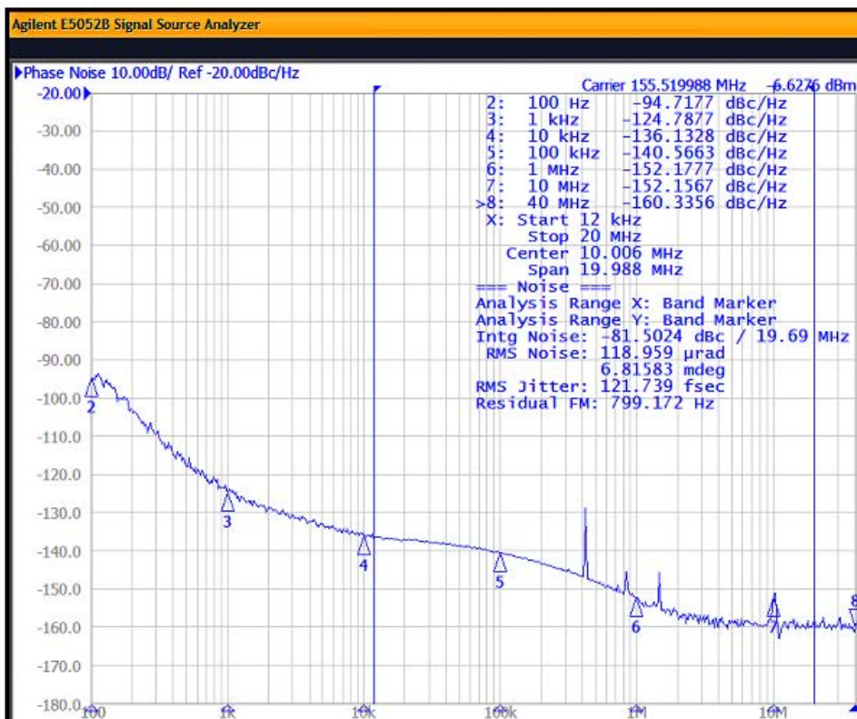
Figure 8.3. Input = 25 MHz; Output = 155.52 MHz, 2.5 V LVDS
