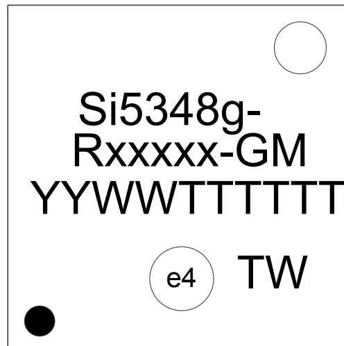
Figure 12.1. Si5348 Top Marking
