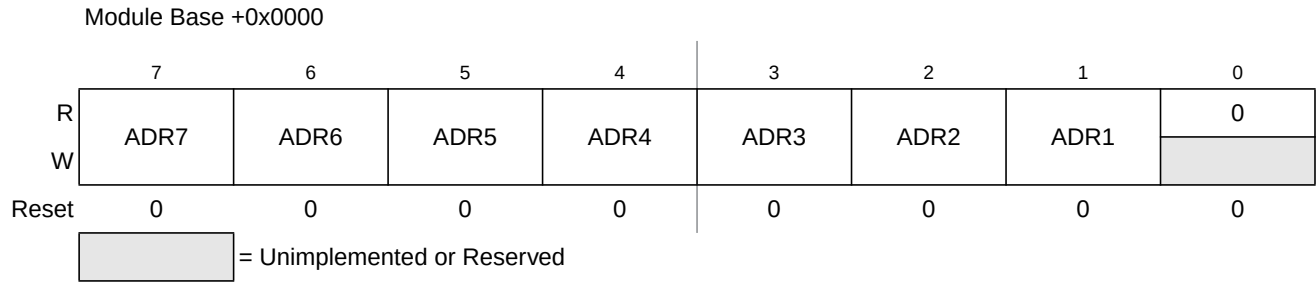
Figure 13-3. IIC Bus Address Register (IBAD)
