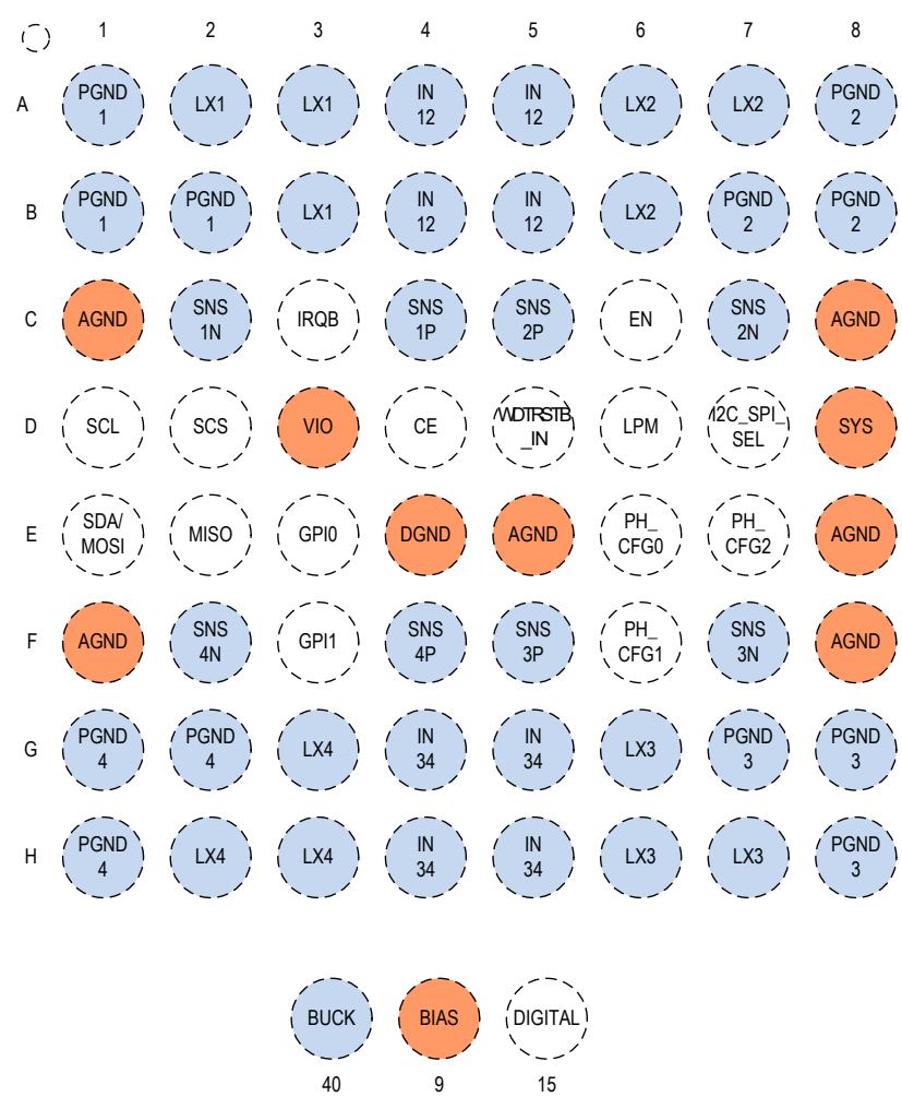
64 WLP (8 x 8 BUMP ARRAY, 0.4MM PITCH) *TOP VIEW = WAFER BACK-SIDE VIEW (BUMPS ARE NOT VIEWABLE)
