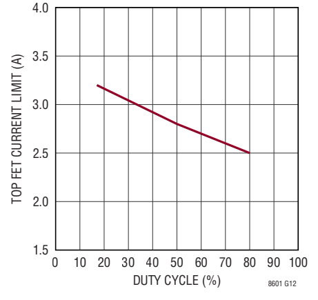
Channel 3 Peak Current Limit vs Duty Cycle
