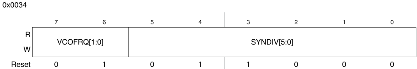
Figure 4-4. S12CPMU_UHV Synthesizer Register (CPMUSYNR)
