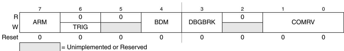
Figure 6-3. Debug Control Register (DBGC1)
