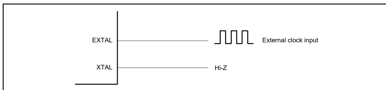
Figure 9.5 Equivalent circuit for external clock
