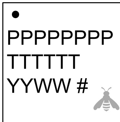
Figure 8.3. QFN24 Package Marking
