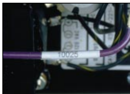
Immediately apply self-laminating labels
