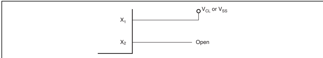
Figure 5.17 Pin Connection when not Using Subclock
