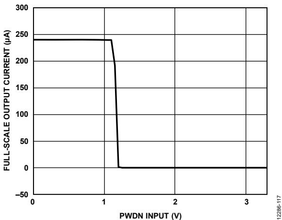
Figure 17. Full-Scale Output Current vs. PWDN Input
