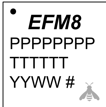
Figure 7.3. QFN28 Package Marking
