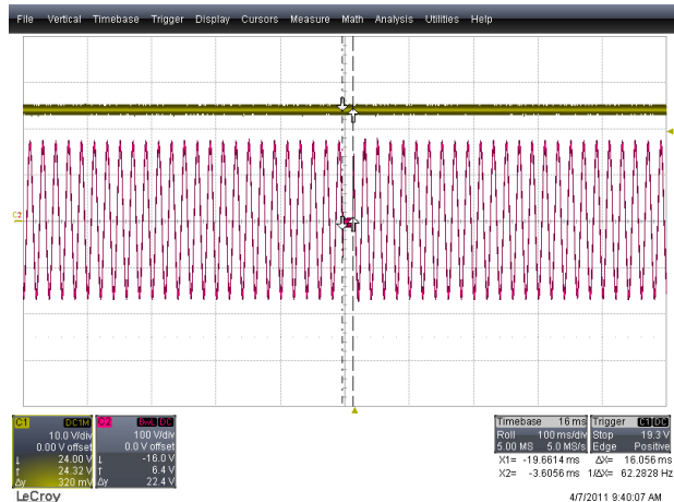
Figure 10: AC drop out 16ms (100 ms/div) CH1: V o (10 V/div) CH2: V in (100 V/div)
