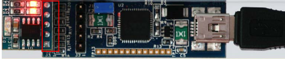
Figure 3-5. Demonstration Board and Bridge Connection
