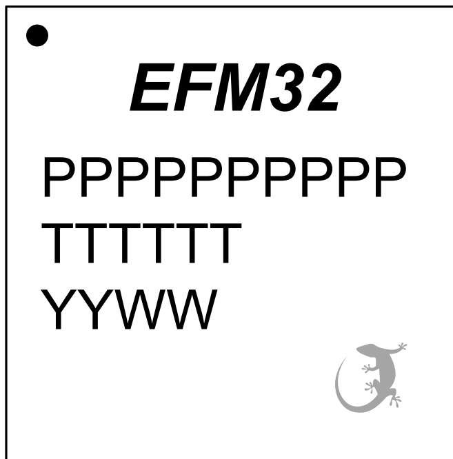
Figure 7.3. BGA125 Package Marking
