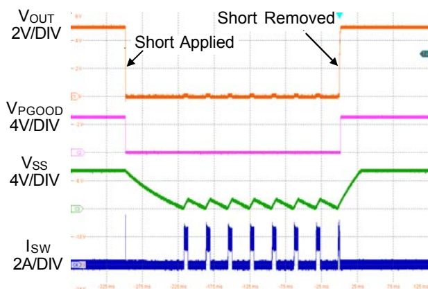
Figure 3. Short Circuit Protection and Recovery
