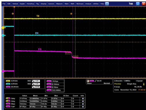
Figure 9-4. CQ in Current Fault Auto Recovery, Low Side Mode
