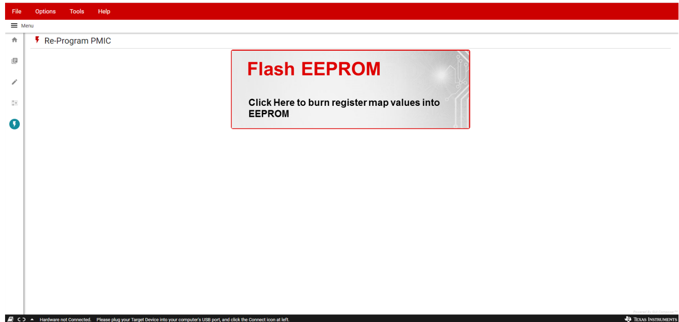
Figure 6-13. TPS6503xx-Q1 GUI Re-Program PMIC Page
