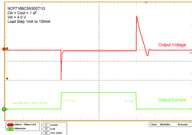
Figure 17. Load Transient Response
