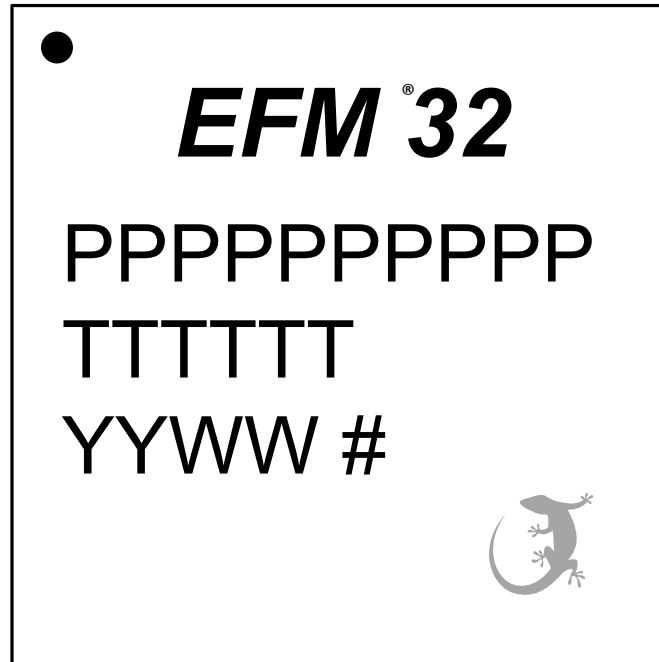
Figure 7.3. QFN40 Package Marking
