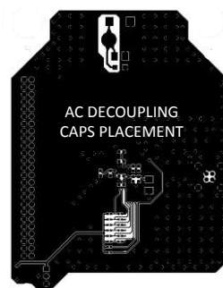
Figure 33. Example DS90UR241-Q1 EMC Layout
