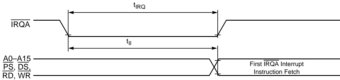
Figure 3-17 Recovery from Stop State Using \overline{IRQA} Interrupt Service
