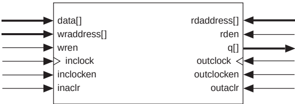
Figure 14-4. Simple Dual-Port Memory Note (1)
