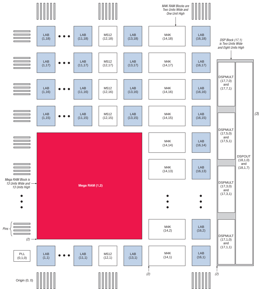
Figure 3–2. Stratix & Stratix GX Architectural Elements Note (1)
