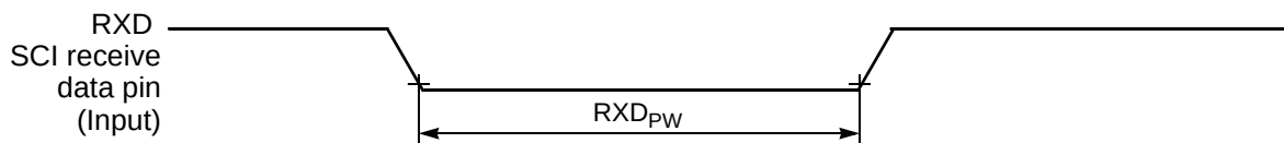
Figure 10-16 RXD Pulse Width
