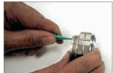
Plastic tool with contact in proper position.
