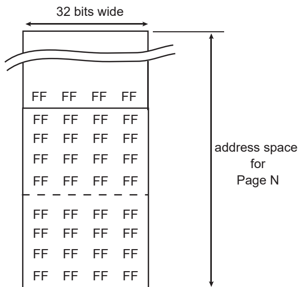
Step 1: Flash array after page erase
