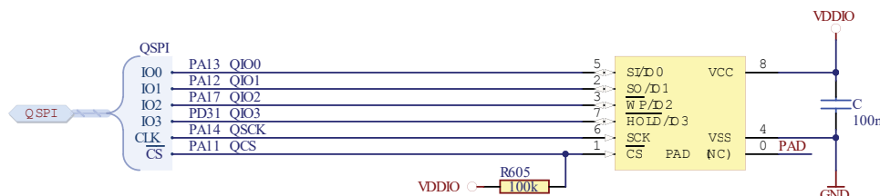
Figure 59-5. Schematic Example with QSPI Data Flash
