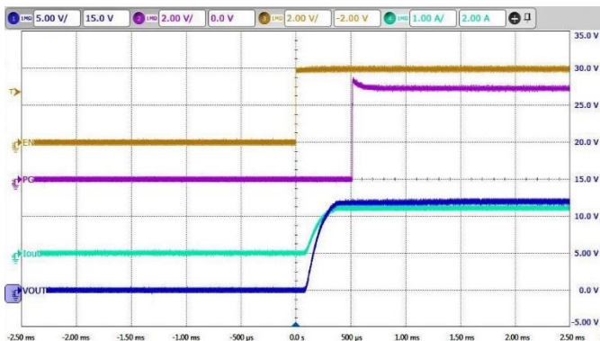
Turn On Response V_{IN} = 12V , V_{CC} = 5V , V_{EN} = 0V to 5V , R_L = 10\Omega
