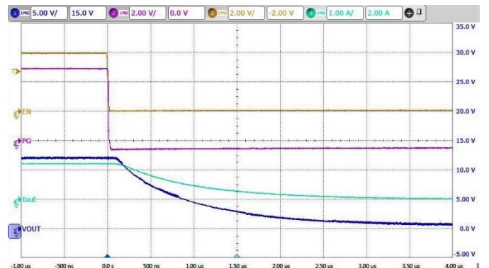
Turn Off Response V_{IN} = 12V , V_{CC} = 5V , V_{EN} = 0V to 5V , R_L = 10\Omega
