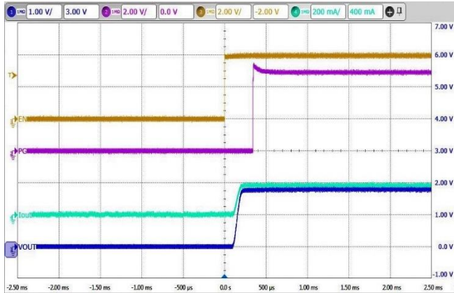
Turn On Response V_{IN} = 1.8V , V_{CC} = 5V , V_{EN} = 0V to 5V , R_L = 10\Omega
