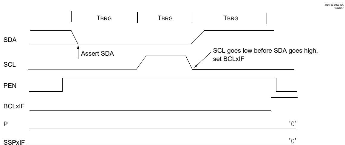
Figure 28-40. Bus Collision During a Stop Condition (Case 2)
