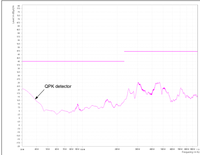
Figure 9-8. CISPR 32 Class B Radiated Emissions: Horizontal Polarization
