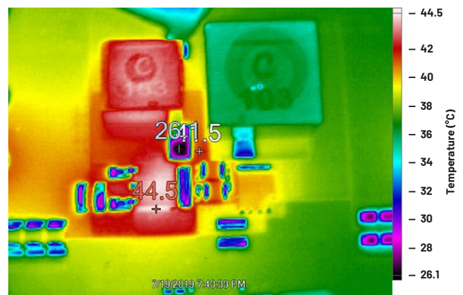
Figure 5. Thermal image of the 4-quadrant converter power train in load (reverse current) mode. A 4.5 A current flows from V_{OUT} terminals to V_{IN} from a 12.5 V source at V_{OUT} .
