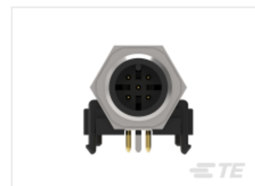
TE Part # 4-2172081-2 M12.MALE.PNLREAR.AC CODE.5P.PCBSTD.RA.SHLD
