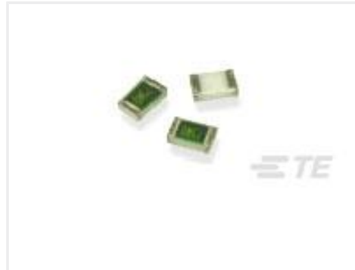
TE Part #1676296-2 RN 0805 2K8 0.1% 10PPM 1KRL
