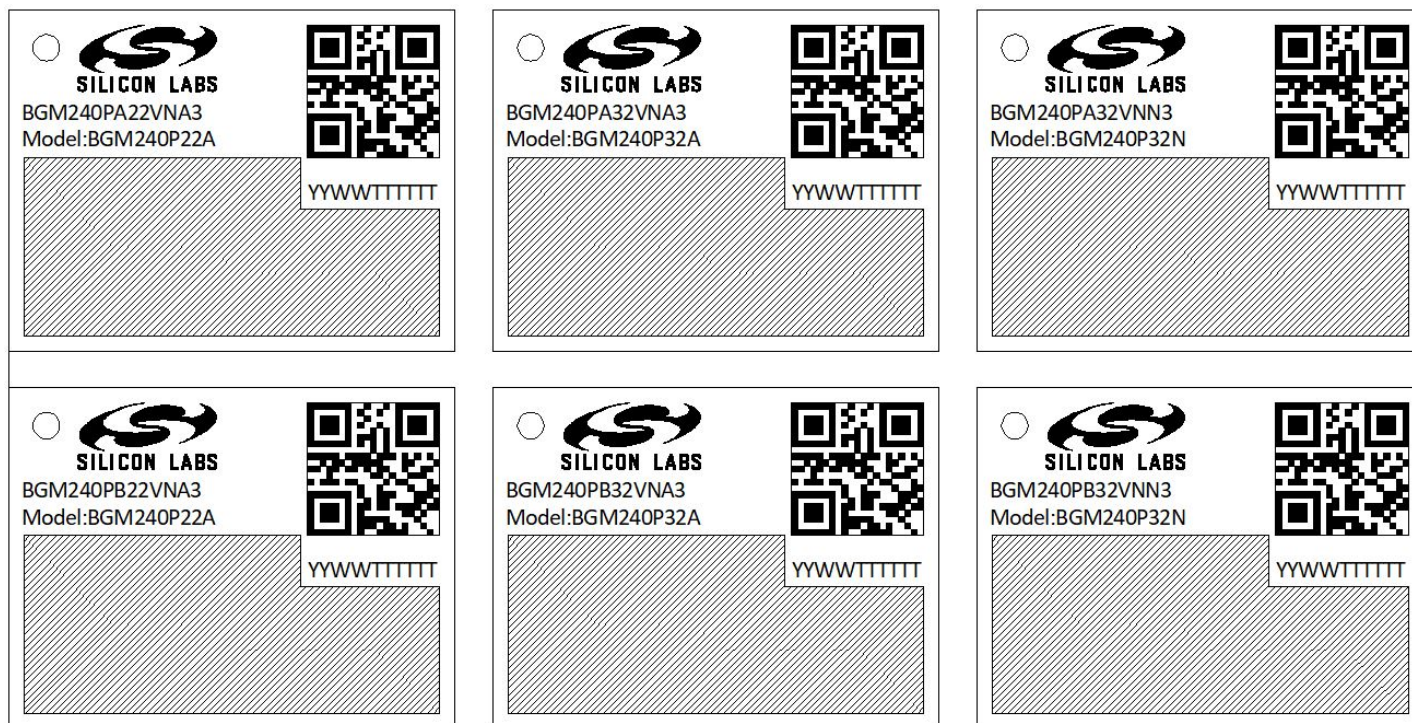
Figure 8.4. BGM240P Top Marking
